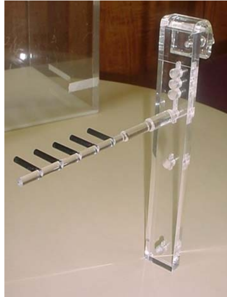
Figure 5: New PQRT TLD Postal System.
