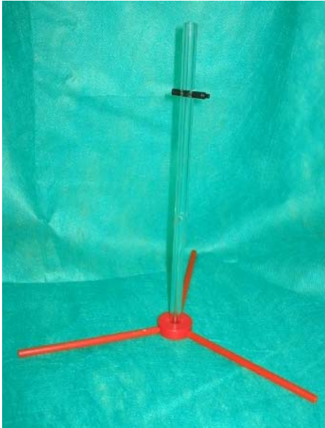
Figure 4: IAEA TLD Postal System.
